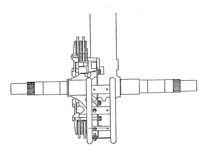
7.6 Place another 30-204 brake assembly on a flat surface, cylinder side up, supported by 2 x 4's as before, and install a 139-19101 bracket as per Section 7.4.
