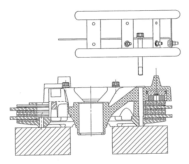
7.5 Slide the brake/bracket/manifold assembly onto the strut as shown. Make sure that the hot air manifold connection lines up with the hot air hose connection.
