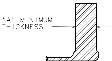
Figure A2 – Disc Thickness Measurement
