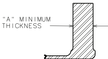
Figure A2 – Disc Thickness Measurement
