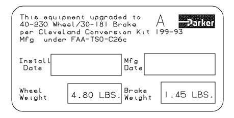
NOTE: If Wheels and Brakes have been retrofitted to 30-181 per Kit 199-93, locate nameplates 166-12500, one each on the Brake and Wheel and scribe an "A" in location shown below.
