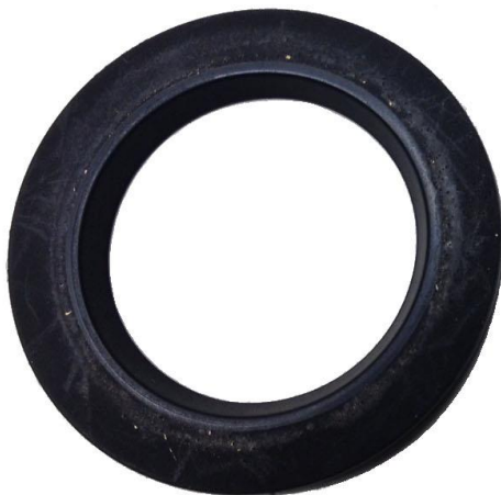
MAXIMUM VARIATION: COMPLETE COVERAGE OF THE METAL PART OF THE SEAL.
