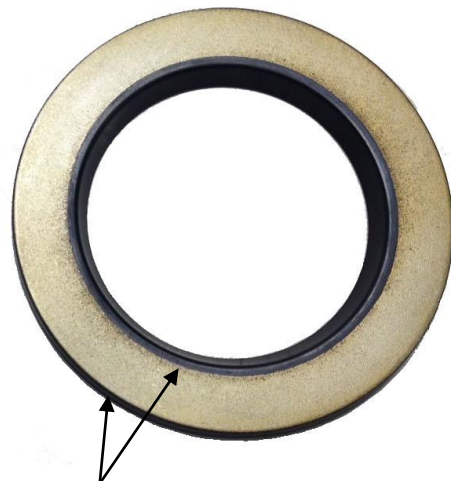
MINIMUM VARIATION: CONDITION EXTENDS OVER ONTO THE METAL PART OF THE SEAL AROUND THE I.D. OR O.D.
