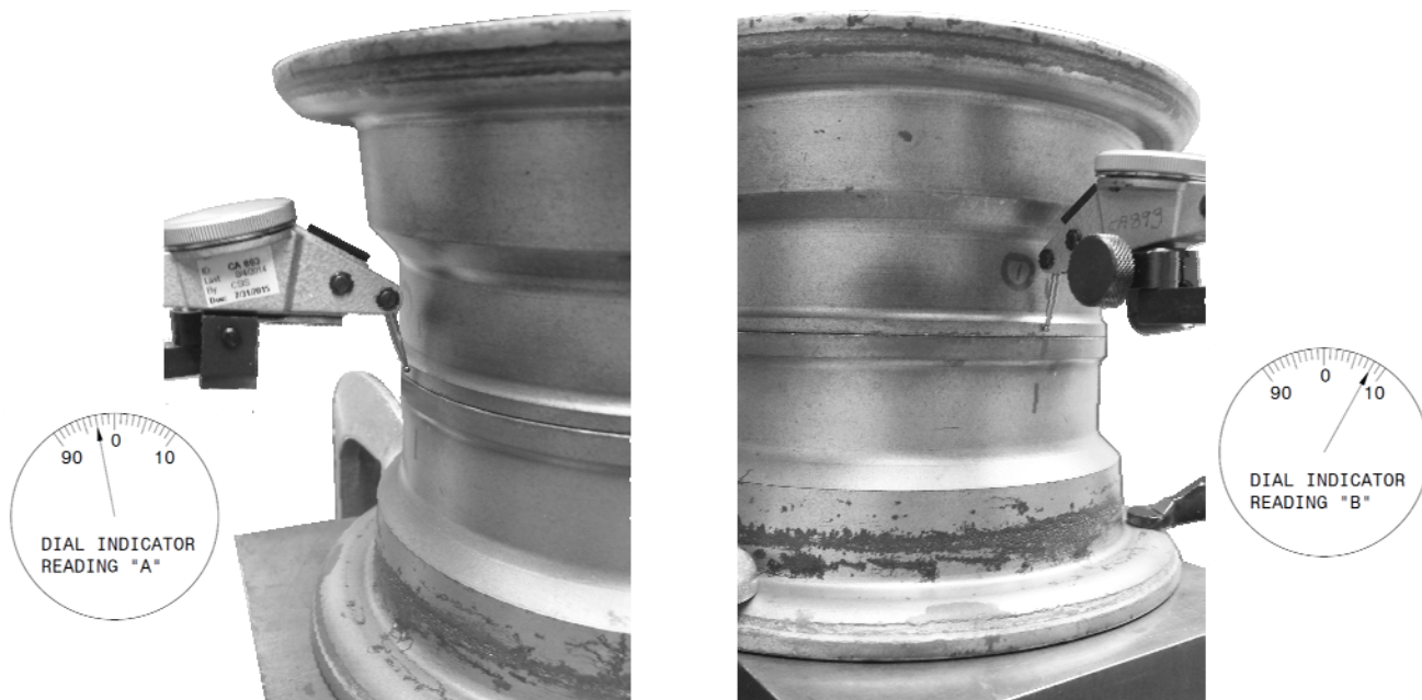
Figure 9 Dial indicator reading, example
