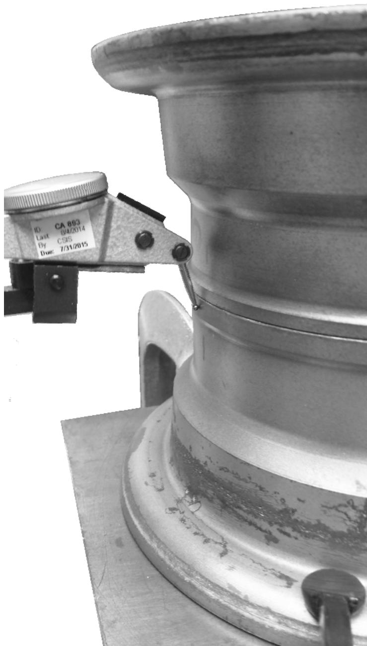
Figure 7 Setup the first position of the dial indicator
