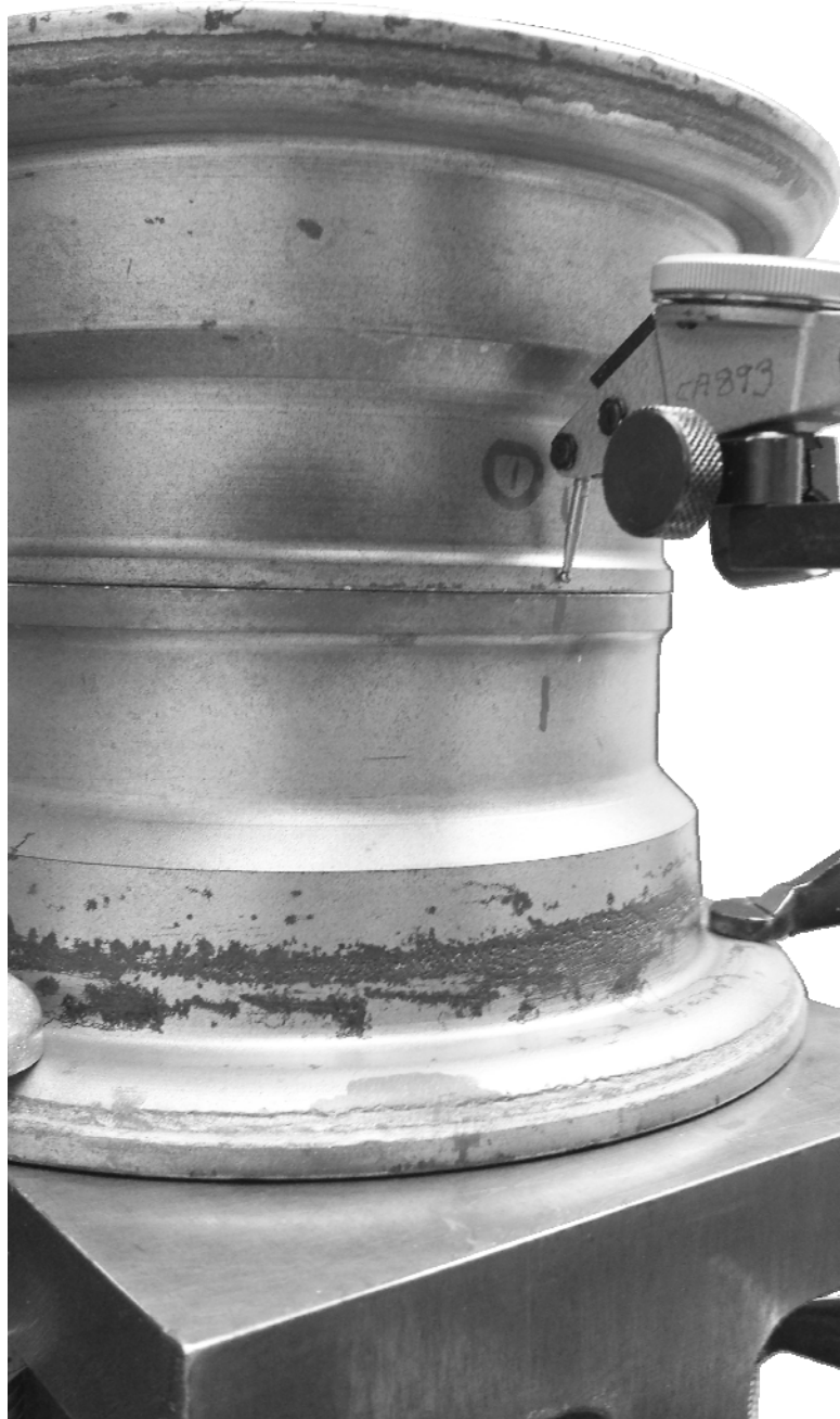
Figure 8 Setup the second position of the dial indicator
